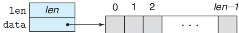
Figure 5.3 Vector abstract data type. A vector is represented by header information plus array of designated length.
